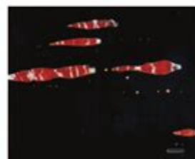
Fig. 3 Cuprous oxide in high-pitch arsenical copper (hot extruded and cold drawn) viewed in dark field, revealing the classic ruby-red color. Magnification bar is 10 \mu m long.
