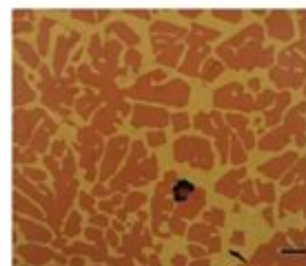
Fig. 2 Microstructure of as-cast Au-22%Al showing the "purple plague," AuAl 2 intermetallic, needles, surrounded by the Al-AuAl 2 eutectic after polishing to a 1 \mu m finish. Magnification bar is 50 \mu m long.
